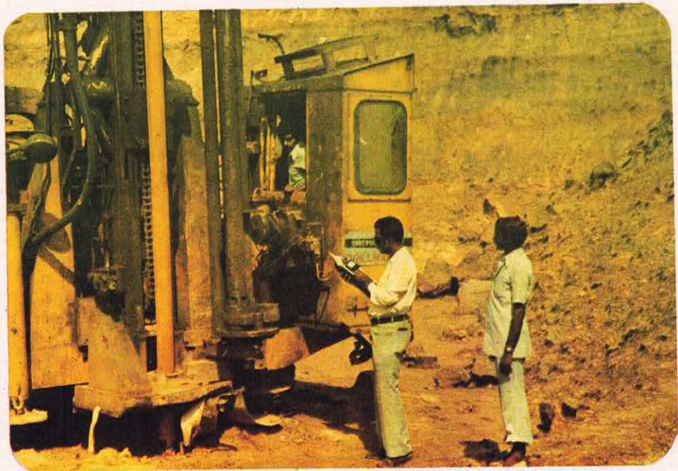
Noise Level Measurements in Drilling Operation in an Opencast Coal Mine (SE/2)
